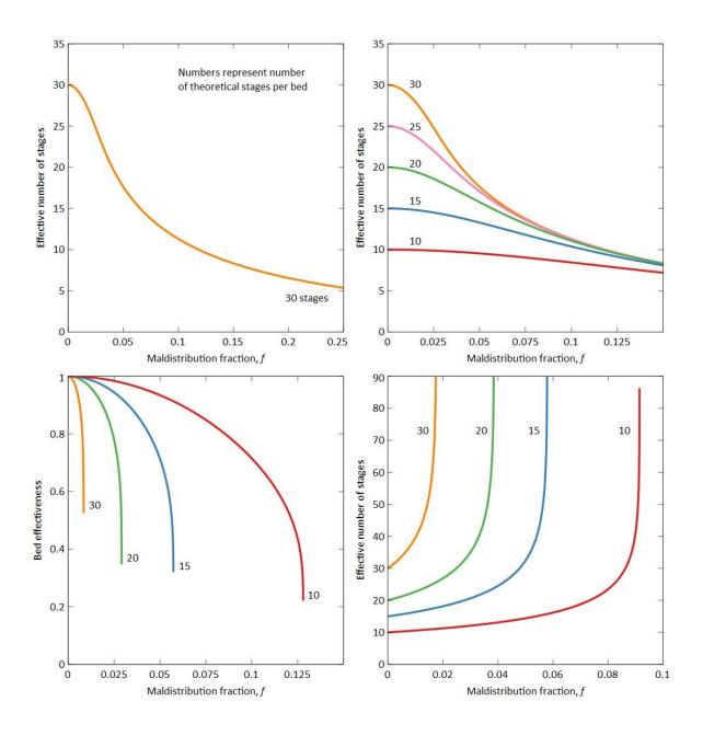
Note the vertical asymptotes; these correspond to the maximum value of f above which no increase in the number of stages can provide the required separation.
